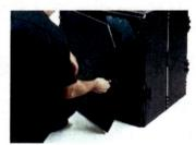
5. Follow local procedures to remove the tamper seal from the Verity Scan handle, if applicable. Unlock the case (if locked). Open the case and remove the power brick and power cord from the storage compartment. Close the compartment and case.
