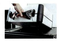
3. Reach inside the ballot box and pull the cord down and away from you to lock the lid and the Verity Scan in place. ▶
